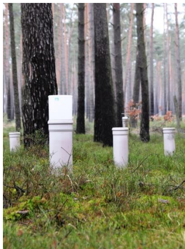
Figure 6-2. Throughfall collectors are distributed across the plot. Throughfall is composed of wet, dry, and occult deposition. However, the exchange process within the tree canopy leads to a depletion of those ions taken up by the trees and an enrichment at the same time due to canopy leaching.
