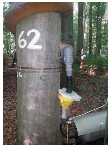
Figure 6-3. Stemflow collectors are permanently installed on the stems to collect any run-off from the branches and stem (here on Fagus sylvatica L.). Stemflow is, compared to throughfall, enriched in ions washed off the bark.
